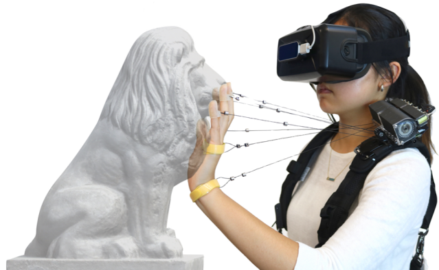
Figure 1. Wireality enables strong, whole-hand haptic feedback for complex objects in VR experiences.
