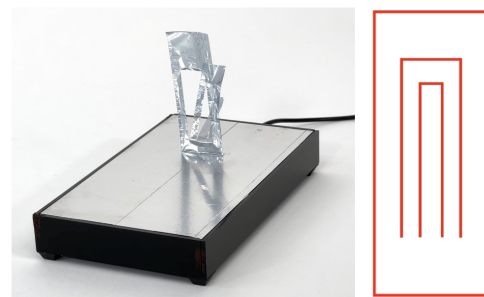
Figure 11: Multiple nested flaps create a repeated geometric elements that repel at different angles.
