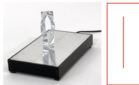
Figure 7: A slit in the film creates two parallel regions which repel to form a loop upon application of electrostatic charge.
