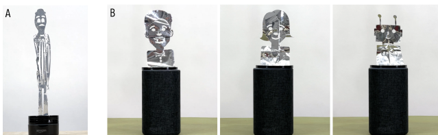
Figure 17: A) We instrumented an Amazon Echo dot with a 40cm pop-up butler, which could activate upon speaking a wake word. B) Users could also personalize their smart speaker agents with inexpensive (<$1) and swap-able avatar pucks, which rest on top of the speaker.
