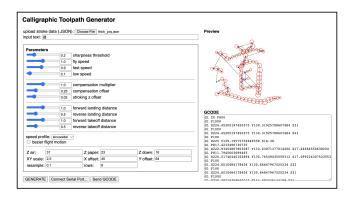
Figure 5: A graphical user interface for previewing the final toolpath of the plotter and adjusting different parameter values to accommodate different brush types.
