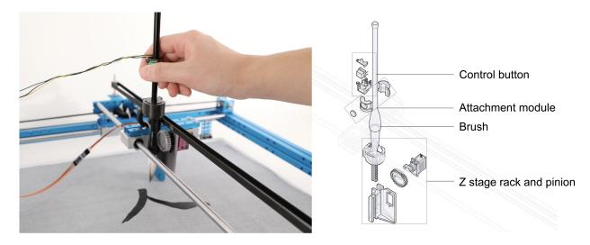
Figure 2: Left: The system's hardware consists of a three-axis plotter. Right: The modified z-axis gantry allows the user to experience continuous movement in the z-direction.
